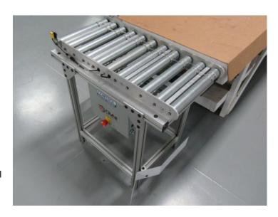
Using additional sensors, the DCA Docking Conveyor can be programmed to discharge or receive multiple loads when docked with a mobile robot. Customer sensors and devices, such as pushbuttons, flashing light beacons, and photo eyes can be wired to the DCA Docking Conveyor to signal the system to perform specific tasks such as calling for a robot to retrieve cargo or to indicate the receipt of cargo.
