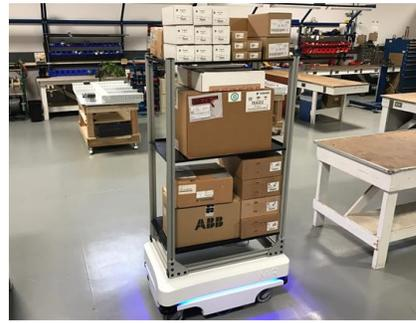
The Omni Automation **TMSU** is a top module that provides adjustable shelving positions for autonomously transporting product, materials, supplies, parts or good in Manufacturing Facilities, Institutions and Warehouses.
