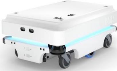
The **MiR100™** is a safe, cost-effective mobile robot that quickly automates your internal transportation and logistics. This 100kg payload robot optimizes workflows, freeing staff resources so you can increase productivity and reduce costs. This robot has a towing capacity of 300kg.
