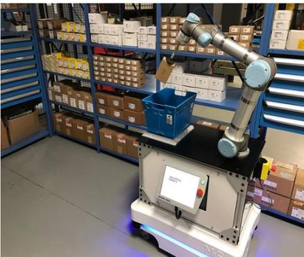
The Omni Automation **TMROR** is a top module with a robotic arm that performs various tasks throughout a facility. These robotic arms utilize a Collaborative Robot with a payload capacity of up to 10 KG. These robots can be used to retrieve product, perform manufacturing tasks, or work along-side humans in industrial manufacturing.
