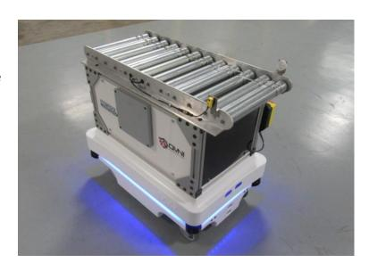
Using additional sensors, the TMRC can be programmed to discharge or receive multiple loads at a single or multiple destinations. These top modules can discharge or receive loads from existing conveyor systems using our **ORP** Interface module. We also offer motorized roller docking conveyors that will communicate directly with the TMRC top modules for a Plug & Play installation.
