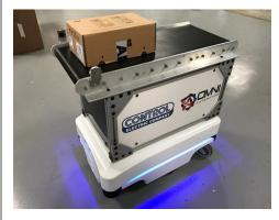
The Omni Automation **TMBC** is a powered belt conveyor that mounts on top of these mobile robots. A mobile robot with a **TMBC** top module can autonomously transport product, materials, supplies, parts or good in Manufacturing Facilities, Institutions and Warehouses
