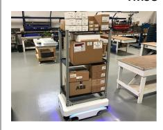
The Omni Automation **TMSU** is a top module that provides adjustable shelving positions for autonomously transporting product, materials, supplies, parts or good in Manufacturing Facilities, Institutions and Warehouses.
