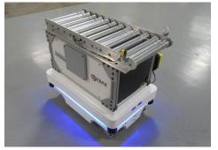
The Omni Automation TMRC is a powered roller conveyor that mounts on top of these robots. A mobile robot with a TMRC top module can autonomously transport product, materials, supplies, parts or good in Manufacturing Facilities, Institutions and Warehouses.
