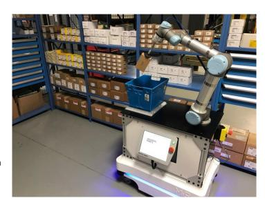
When the TMROR arrives at a docking station the robot communicates with the fixed automation over Wi-Fi or Bluetooth to signal the process to begin. Once the process is completed, the mobile robot is signaled to continue its mission to other locations in the facility.
